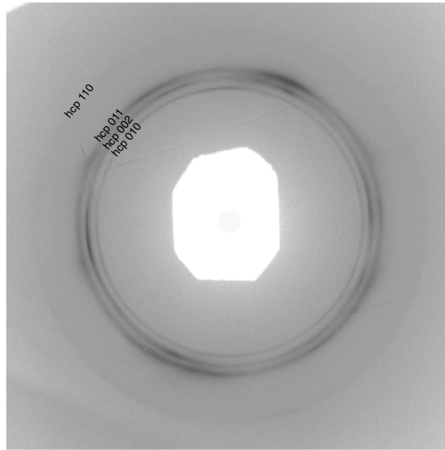
Figure 2. Two-dimensional XRD pattern of \text{Fe}_{0.88}\text{Si}_{0.12}\text{H}_{0.61} at 138 GPa (see text for details).
